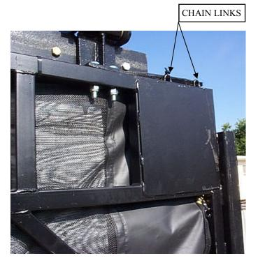
23. FOR TRAILERS THAT ARE SHORTER THAN THE TARP LENGTH, CUT THE TARP AT THE BACK OF THE TRAILER, BUT LEAVE APPROX. 6" to 8" (15cm to 20cm) EXTRA MATERIAL. FOLD OVER THE EXCESS MATERIAL, AND USE THE ALUMINUM COVER STRIPS WITH SELF DRILLING SCREWS PROVIDED TO ATTACH THE TARP TO THE REAR LID AS SHOWN BELOW. **NOTE:** COVER STRIPS ARE SHOWN BELOW FOR PLACEMENT, TARP IS NOT SHOWN.
