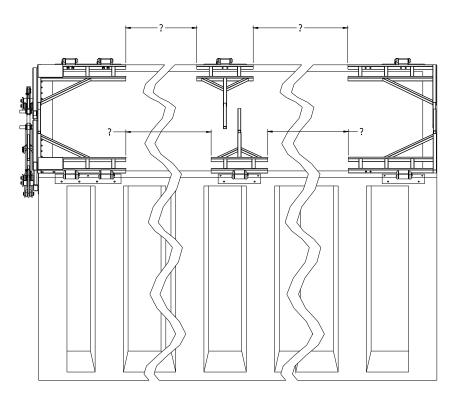
17. ADD 8" (20.3cm) TO EACH OF THE (4) MEASUREMENTS TAKEN IN STEP #10. THIS WILL BE THE LENGTH OF THE LADDER SECTIONS BETWEEN THE LIDS. WELD THE "H" CONNECTORS AND LADDERS ON THE GROUND AS SHOW BELOW. THE LADDER SECTION MAY NEED TO BE CUT, AND/OR EXTRA "H" CONNECTORS AND LADDERS (SUPPLIED) MAY BE USED TO OBTAIN THE DESIRED LENGTH.
