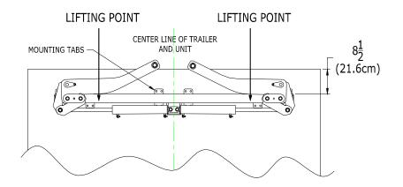
**NOTE**: IF FRONT WALL OF TRAILER IS THIN ALUMINUM OR STEEL, USE SUFFICIENT BACKING PLATES INSIDE OF TRAILER TO SUPPORT THE UNIT. **NOTE**: IF TRAILER HAS A ROUND OR 45 deg FRONT CORNER YOU MUST SUPPORT THE FULL ACTUATOR
